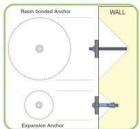
Torque controlled expansion anchors are far superior in performance than 'hammer- in' screw fixings, being typically in excess of 10x stronger for the same diameter.
